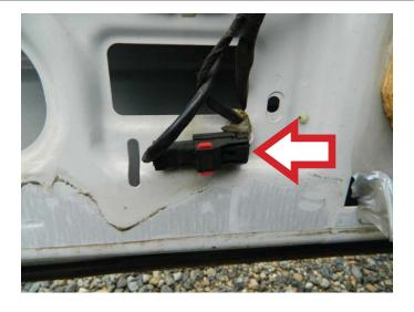
**STEP 4:** Temporarily install the master power window switch so that you can lower the door glass to meet the attaching mounts on the window regulator.
