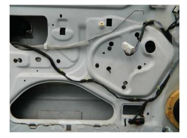
STEP 6: Remove the water vapor barrier.
