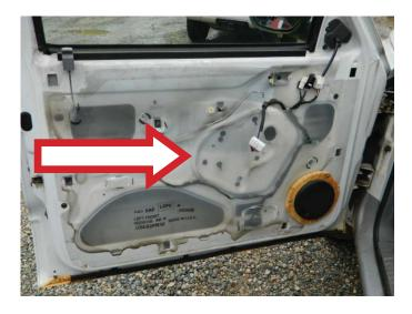
**STEP 5:** Install the water vapor barrier.
