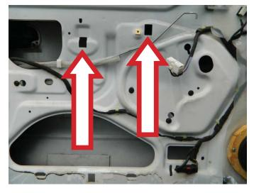
STEP 4a: Attach the window glass to the window regulator.
