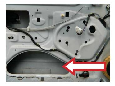
**STEP 10:** Remove the window lift motor attaching hardware. **WARNING:** USE EXTREME CAUTION WHEN REMOVING THE WINDOW LIFT MOTOR FROM THE WINDOW REGULATOR, THE PRETENSIONER SPRING IS UNDER PRESSURE. IT IS ADVISED THAT YOU REMOVE THE PRETENSIONER SPRING FIRST BEFORE LOOSENING THE WINDOW LIFT MOTOR.
