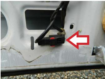
**STEP 7:** Disconnect the window lift motor connector.
